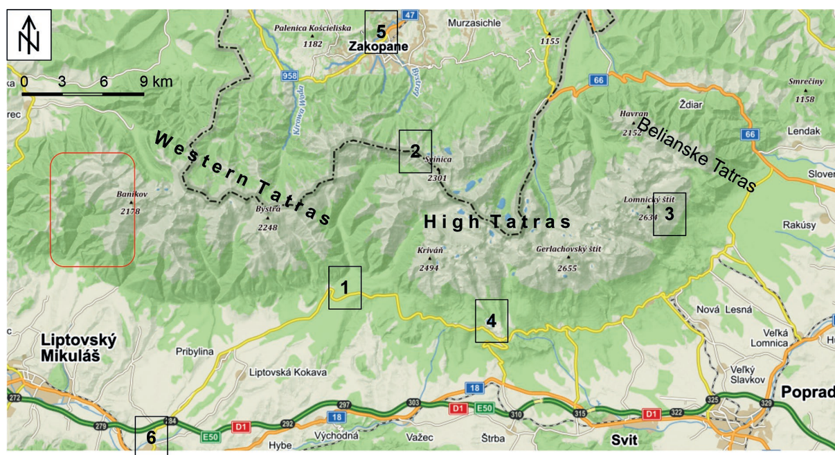
Fig. 2.5. The Tatra Mountains (based on www.mapy.cz ). The rounded rectangle on the left marks the Jalovecký Creek research catchment (area 22.2 km 2 , mean elevation 1500 m a.s.l.); 1 – gauge on the Belá river (Podbanské) which has the longest record of annual runoff among the small mountain catchments of the Tatra Mountains (since 1895); 2 – the high mountain meteorological station Kasprowy Wierch (Western Tatra Mountains, 1991 m a.s.l., windward position, established in 1937); 3 – the high mountain meteorological station Skalnaté Pleso (High Tatra Mountains, 1778 m a.s.l., leeward position, established in 1939); 4 – meteorological station Štrbské Pleso (High Tatra Mountains, 1354 m a.s.l., leeward position, established in 1902); 5 – meteorological station Zakopane (the foothills, 855 m a.s.l., windward position, regular data since 1911); 6 – meteorological station Liptovský Hrádok (the foothills, 640 m a.s.l., leeward position, established in 1881).
